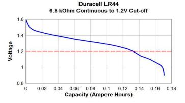
Delivered capacity is dependent on the applied load, operating temperature and cut-off voltage. Please refer to the charts and discharge data shown for examples of the energy/service life that the battery will provide for various load conditions.
